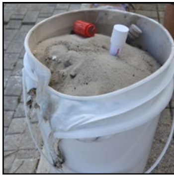
Wet sand pails were at each flare station to extinguish flares; this bucket melted under the heat
