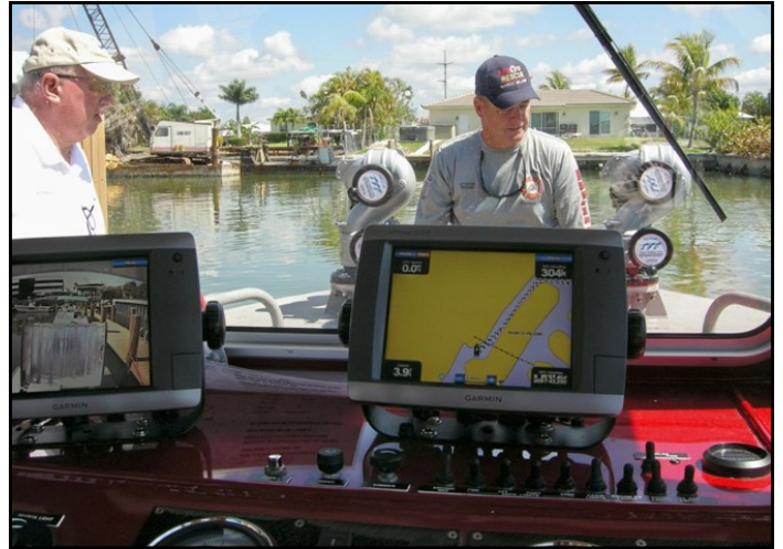
Cdr Carl Thieme, SN and Capt. Tom Bogan; new boat designed to fight fires while shooting 1500 gal. of water per min. through two bow mounted nozzles aimed at burning vessels or fires on shore.
